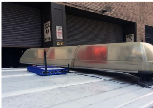
Figure 6 - IoT Data Aggregator on Roof of Vehicle
